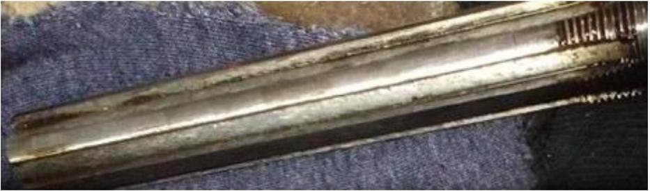
All the parts were degreased and cleaned using white spirit. I was somewhat amazed at the amount of casting sand that had been left in the castings, this can all wash down onto and into the bearing surfaces causing accelerated wear (possibly a Chinese design feature 😊).
