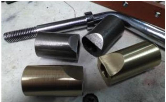
the originals. The bushes were then put in the lathe faced off to length, drilled and taped as required. Photo 5 (previous page) shows the completed bushes and the original cast iron ones. The shiny area on the grey ones shows the original clamping area.
