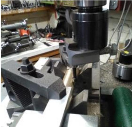
A length of bronze was put in two vee blocks and clamped in the machine vice. Clamping the bar in the machine vice ensured that the bar was aligned to the table axis. The bar was then clamped down to the table above the vee blocks. (the set up and machining is shown in Photo 4 left. The bolt sticking out of the back of the boring head is to reduce the boring head imbalance).
