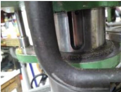
There was enough clearance between the housing and the spindle to allow a bush to be inserted, to block off these two slots. I machined a steel bush to be a press fit, I also put in a small 1/8" oil hole to enable the bottom spindle bearing to be lubricated. This was pressed in so that the oil hole aligned with the top of the original slot (Photo 2 above).
