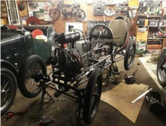
The project started when I came across a 300cc Norman generator engine and an old chassis, meant for some kind of motorised cart. I then started to collect 19inch motorcycle wheels and a gearbox from an agricultural rotorvator. I found lots of other useful items, such as parts of outboard motors,
