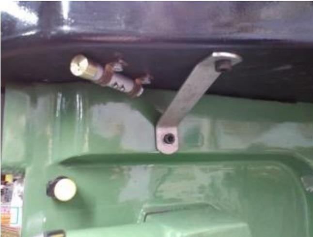
The laser pen was mounted on the mill out of the way on the bottom of the guard. The guard proved to be too flexible hence the stainless bracket (photo 6 left). The brass shield with a small hole in it is to reduce the diameter of the laser beam. I suspended a plumb line from the ceiling at the other end of the workshop and align to
