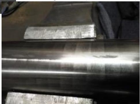
Whilst the mill was stripped apart, I had noted that the spindle locking mechanism, that caused the bruising, consists of two cast iron bushes that have a 45° angle cut on the end. These are forced together by the locking handle, clamping the spindle. Because of the straight angular cut, this produces a ridiculously small area that clamps, hence the damage. I decided to make up replacement clamping bushes from Phosphor bronze with a curved clamping area the same radius as the spindle housing.
